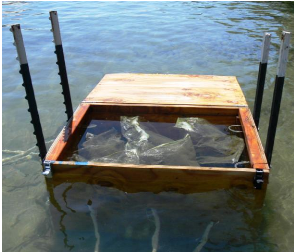
Figure 21: Deer Lake groundwater collection box.
