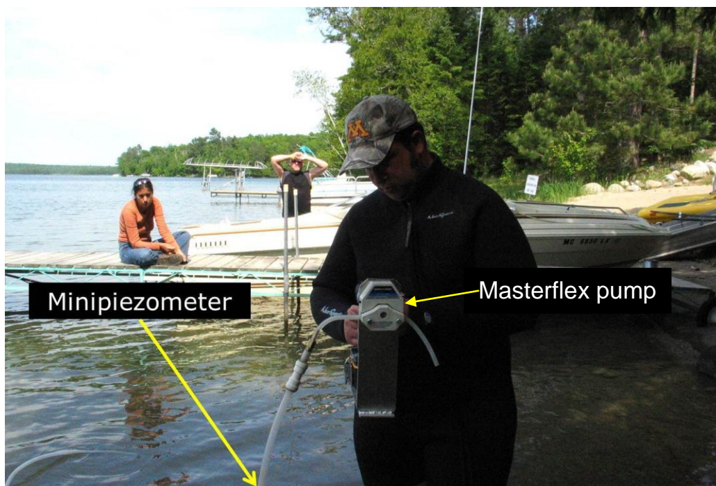
Figure 14: Using Masterflex pump to collect groundwater sample from minipiezometer.
