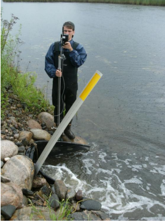
Figure 94: ICSWCD intern measuring discharge at highway 169 storm water retention pond.
