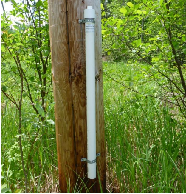
Figure 5: Air-pressure-compensated Hobo data logger
